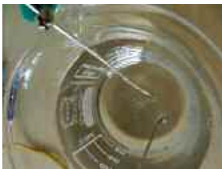
As soon as a closed circuit exists, tiny bubbles appear at the cathode.
