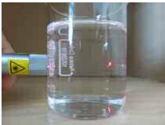
The beam of the laser pointer cannot be seen, since the water contains no colloidal particles.
