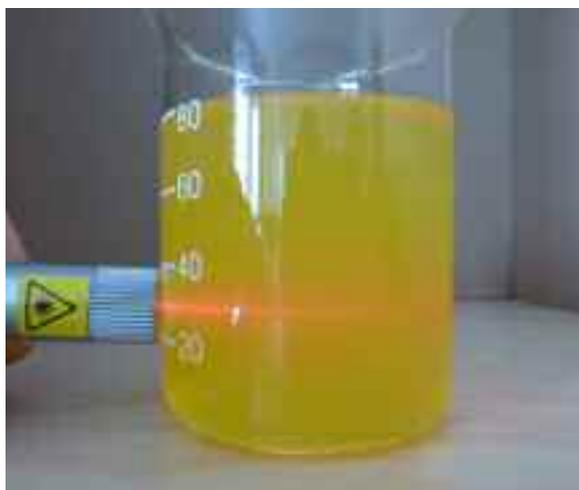
The visible beam of the laser pointer proves that nano-scale colloidal particles are present in the solution.
